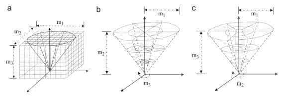
**Fig. 5.** Different quantisation models. (a) Model  $M_{\#}$ , (b) Model  $M_{\otimes}$  and (c) Model  $M_{\odot}$ .
