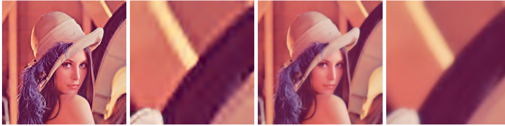
(a) JPEG2000 31.19dB. (b) JPEG2000-CIWaM 27.57dB. Fig. 3 Examples of reconstructed images of Lena compressed at 0.9 bpp.
