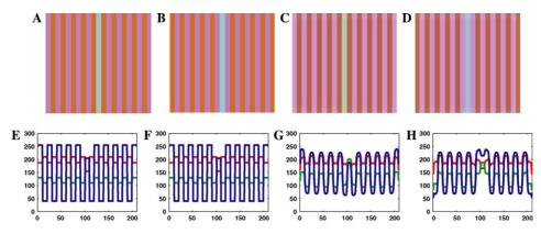
Fig. 8. (A,B) Examples of two images presenting important assimilation effects. (C,D) Previous images transformed by Spatial-CIELAB. (E–H) are the RGB profiles of images (A–D), respectively.
