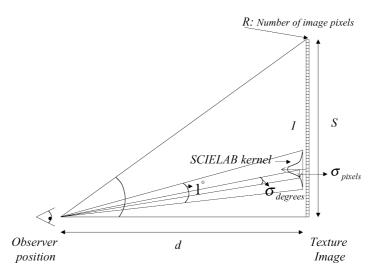
Fig. 6. General scheme for unit conversion from visual angle to image pixels.
